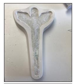
Cover the cavity with F3 Medium Clear frit until the mold holds a total of 72 grams of glass.
