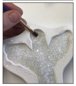
Gently sweep the frit away from the post with a paint brush or similar tool to prevent burrs. Fire the mold using the schedule found in table 1.
