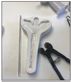
Fill the icicle portion of the cavity with a clear rod cut to size and/or thin strips of clear sheet glass.
